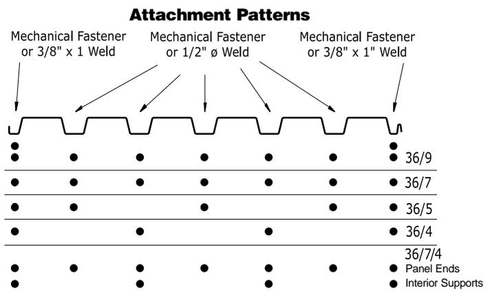
Note: Weld sizes are effective not visible. Refer to AISI S100 or AWS D1.3 for additional welding requirements.
