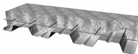
Maximum Unshored Span Gage Single Double Triple 22 7' - 4" 8' - 5" 8' - 7" 21 8' - 3" 9' - 3" 9' - 7" 20 8' - 10" 9' - 10" 10' - 2"
