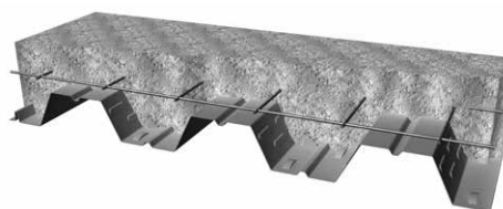
Maximum Unshored Span Gage Single Double Triple Gage Single Double Triple 22 9' - 5" 10' - 3" 10' - 7" 19 11' - 8" 13' - 0" 13' - 5" 21 10' - 3" 11' - 0" 11' - 4" 18 12' - 0" 14' - 2" 14' - 1" 20 11' - 0" 11' - 8" 12' - 0" 16 12' - 8" 15' - 10" 14' - 10"
